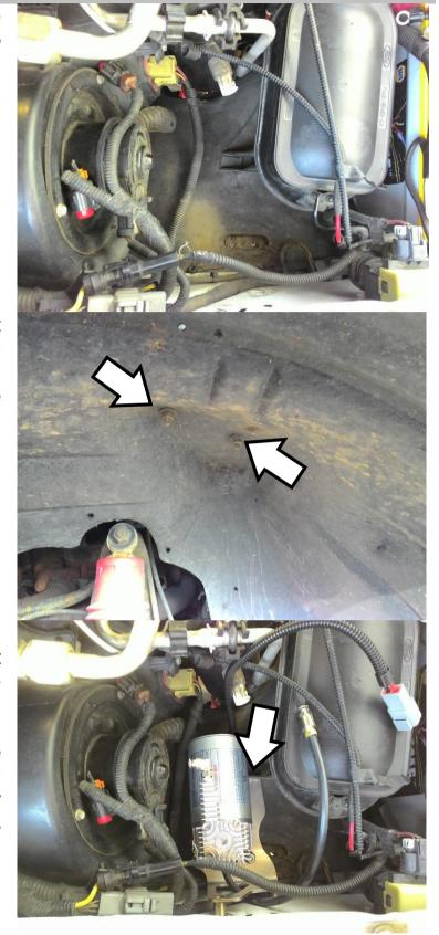
Install the supplied bolts and lock washers to attach the pump bracket to the fender where the vacuum pump previously attached. Reinstall the two 11mm nuts holding the vacuum reservoir.
