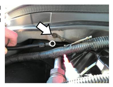
Connect the ring terminal on the red wire to the passenger side positive battery terminal (The negative battery leads should not yet be connected at this time).
