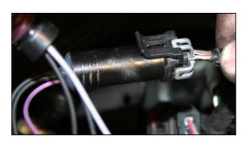
Route the harness away from moving parts or major heat sources and through the firewall to a location under the dash suitable for mounting the brake control module, which will be installed next.
