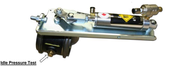
With the BD brake engaged and the engine at idle check the exhaust backpressure using a pressure gauge (such as BD PN 1030050) at the test port on the brake valve.
