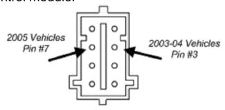
Connect the supplied Pink wire to the **Brake Output** terminal on the control module and the Grey wire to the **VSS In** terminal and route both wires through the firewall.
